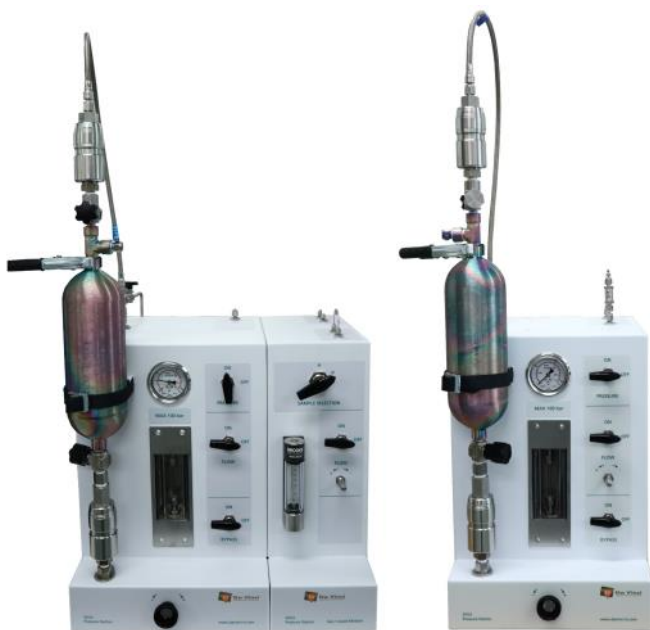
Figure Eight: The DVLS Pressure Station
